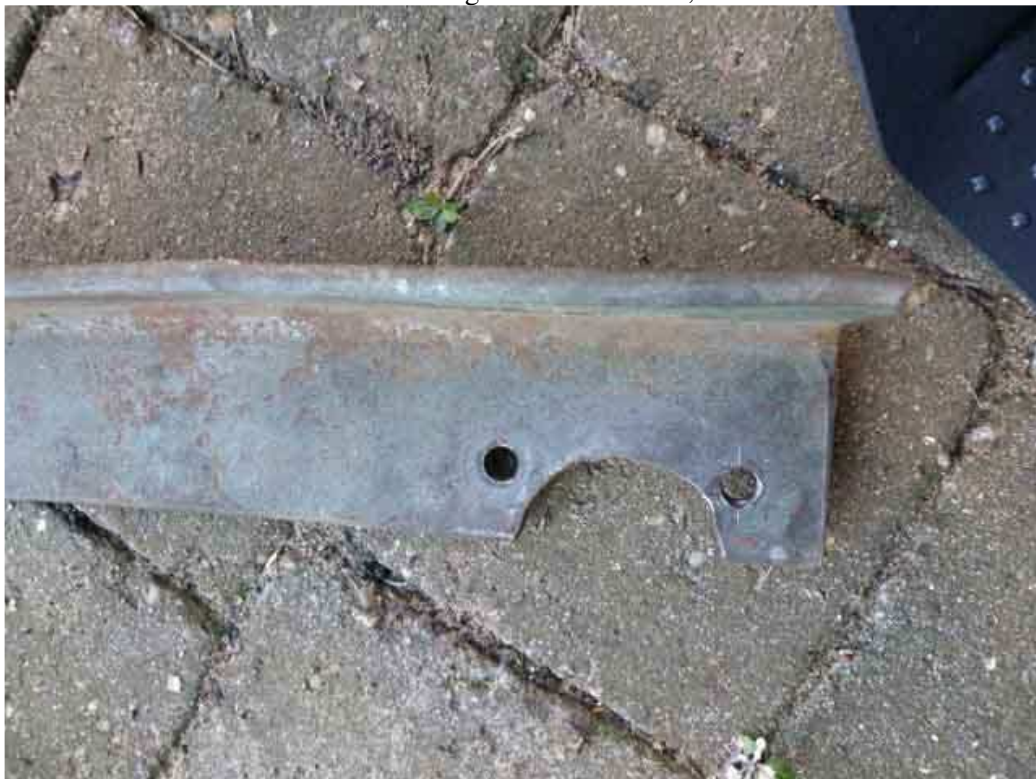
The 'tool' used to hold the drive flange steady while the central nut was undone - a piece of 2 1/2" angle iron, with a curved section cut out and 2 holes. The flange nut is 1 1/8" AF, same as the front hub nuts.
