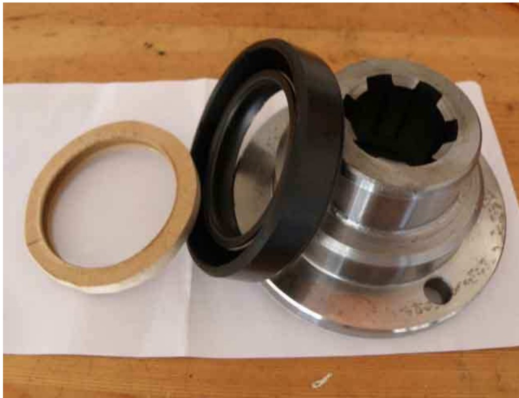
The seal fitted over the flange
